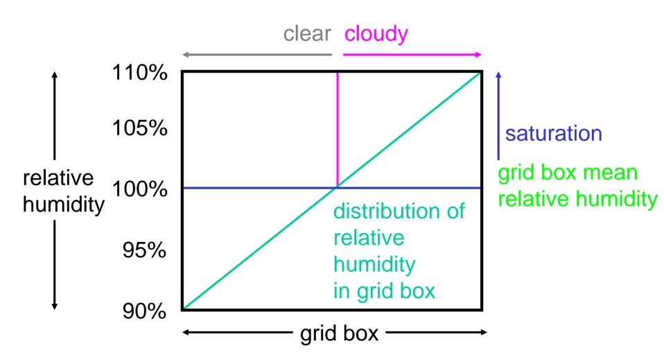
Assuming the previous "triangular" distribution of relative humidity in the grid box, we now have a parameterization for percentage cloud cover C as a function of grid box mean relative humidity RH.
