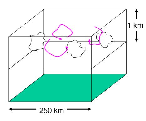
Parameterization is representing the effects of unknown small scale properties from known grid box mean properties
